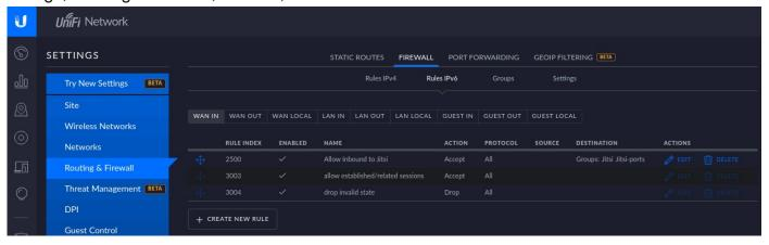
In my exmple below, I have a Jitsi server running on an LXC container on my VLAN 80 network where I have enabled IPv6. This is the inbound IPv6 router rule:
