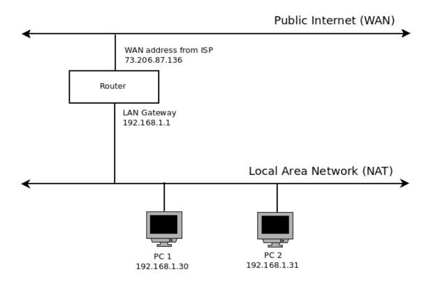
This arrangement works just fine for putting multiple systems on a private network. When PC 1 goes to a website, the 192.168.1.30 address is encapsulated in the outbound packet which is identified by the 73.206.87.136 WAN address. When the website returns its information to 73.206.87.136, the router sees the encapsulated address 192.168.1.30 for PC 1 is where the data should be sent.
